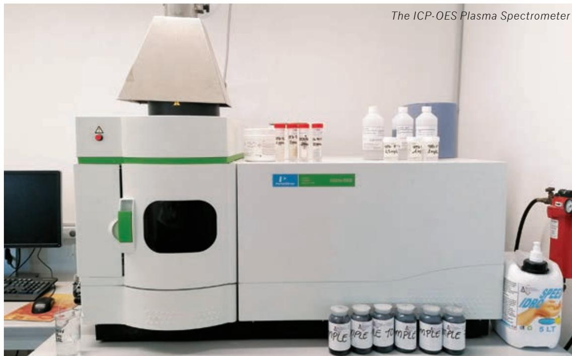
The ICP-OES Plasma Spectrometer
