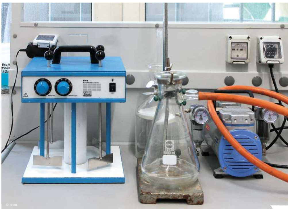
A jar test instrument (left) and a vacuum filtration pump.
