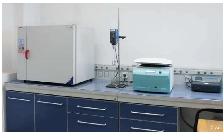
From left to right: a thermostatic heater, a mixer, a spectrometer, and a centrifuge.
